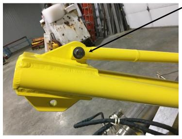
At the other end of the support rod, install a 3/8-16 bolt through the rod and the hole at the end of the boom then tighten.
