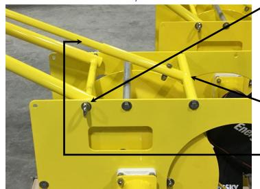
Install two ½-13 eye bolts through the winch side plates on both port and starboard sides into the base of the boom. Tighten the eye bolts until snug and then rotate ½ turn tighter.
